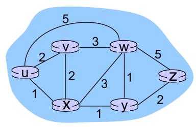
clearly,  $d_{v}(z) = 5$ ,  $d_{x}(z) = 3$ ,  $d_{w}(z) = 3$ B-F equation says:  $d_{\mu}(z) = \min \{ c(u,v) + d_{\nu}(z), \}$  $c(u,x) + d_{x}(z),$  $c(u,w) + d_w(z)$  $= \min \{2 + 5,$ 1 + 3, 5 + 3 = 4 node achieving minimum is next
